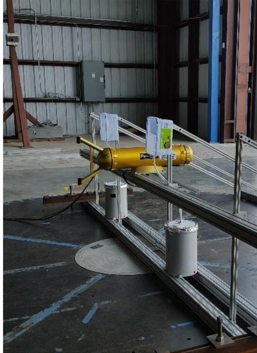
Figure 38. TB3 rain gauge connected to vertical rain collecting bucket
