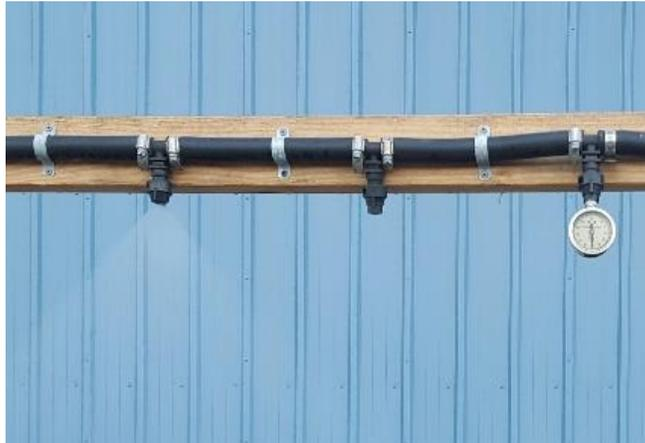
*Figure 32. Pressure gauge installed on the hose*
