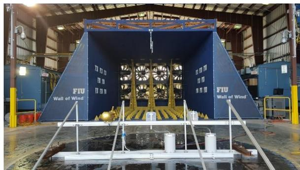
*Figure 24. 12-fan Wall of Wind (WOW)*
