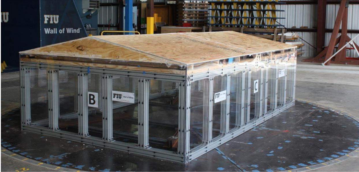
**Figure 1-5 Reduced-Scale Model Building**
