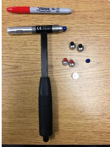
Figure 5. Impulse hammer (PCB model 086C01)
