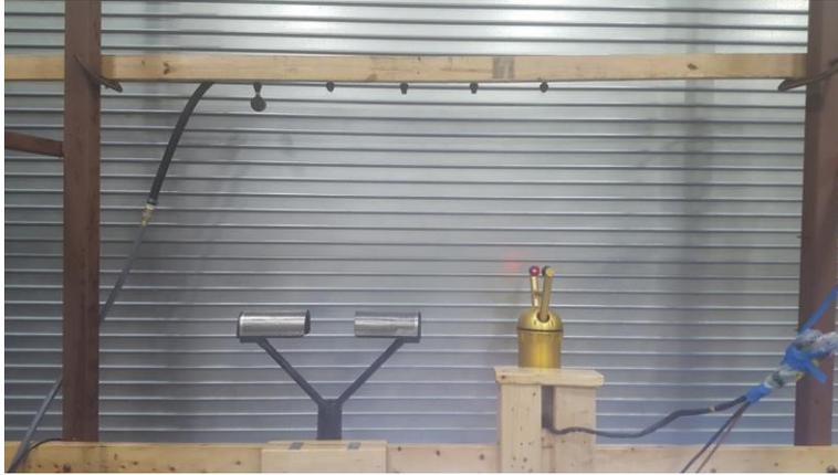
*Figure 28. Droplet measurement using Parsivel and PIP for single nozzle spray in stagnant air*
