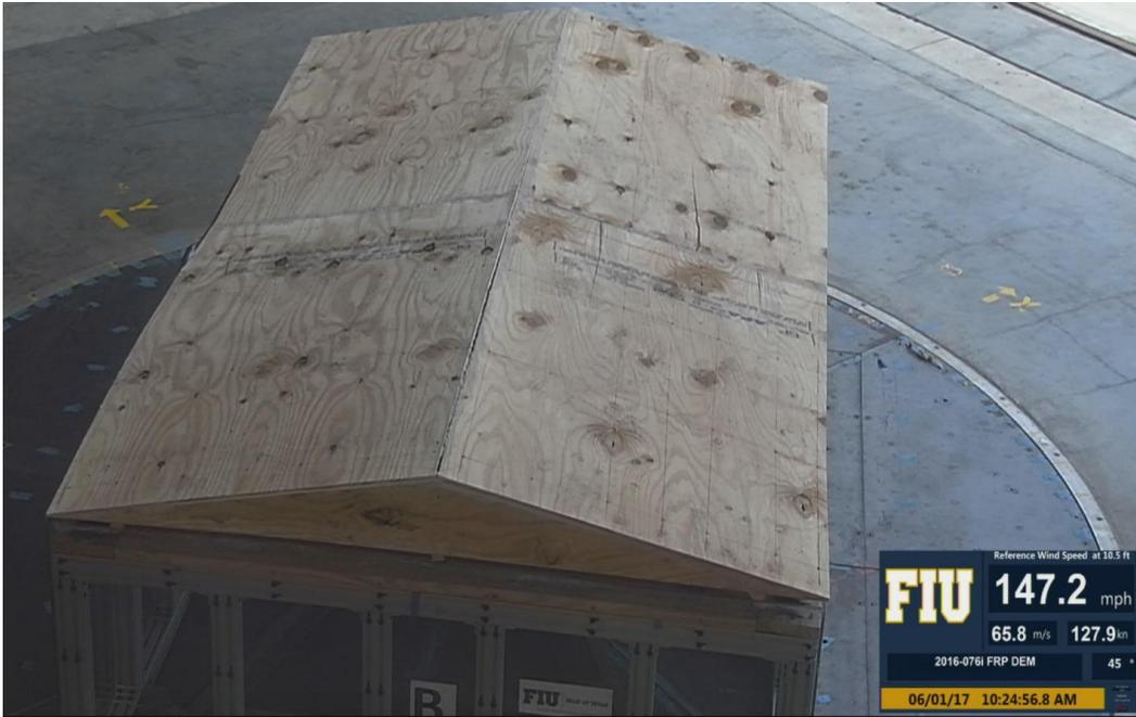
**Figure 1-13 Model before Failure**
