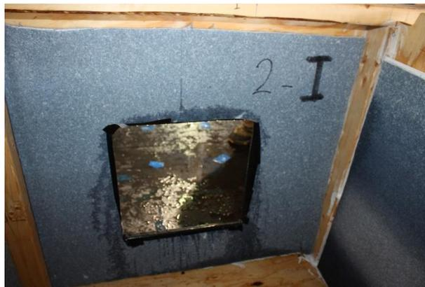
Figure 49. Interior walls covered with water absorbent pads
