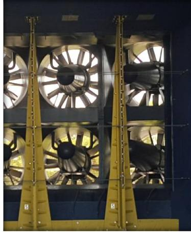
Figure 34. Vertical spires in front of the WOW where the nozzles will be installed on the hoses
