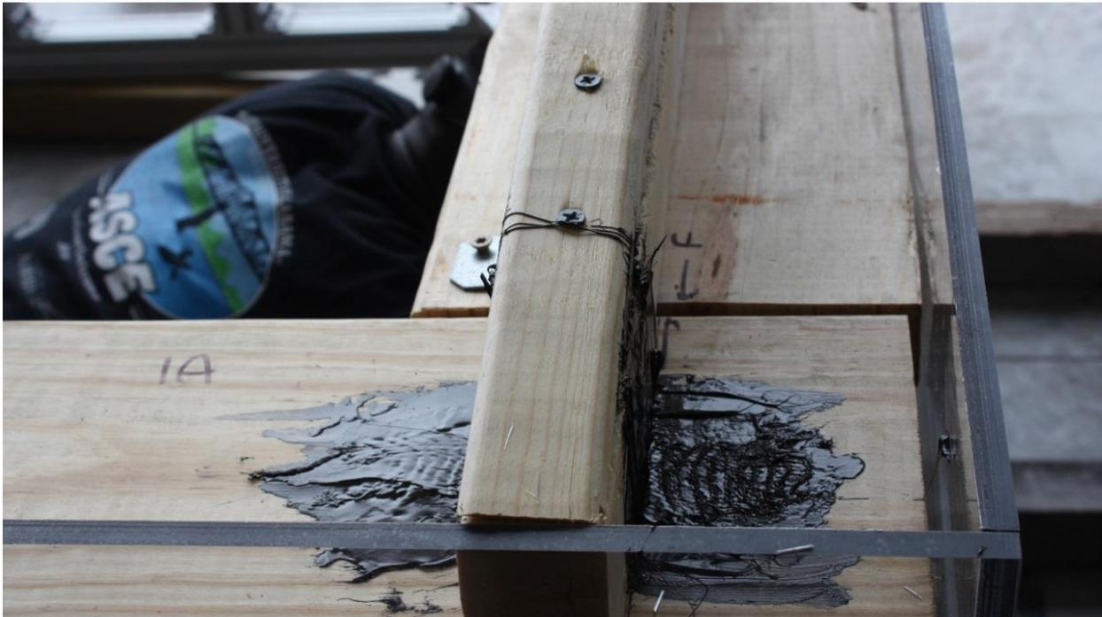
**Figure 1-7 Roof-to-Wall Connection on Each End of the Truss**
